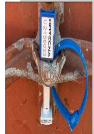
Seal stem is bent. Seal does not lock properly.
